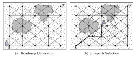
**Fig. 1.** Working of the Navigation Algorithm. The figures show the grid roadmap. Roadmap vertices and sensor nodes are depicted by black dots and gray dots, respectively. The start and goal are denoted by S and G respectively. The gray shaded regions denote fire. Figure (a) shows the generated roadmap. Figure (b) shows the sub-path selected (dotted arrow) within the query area (shown by the circle). The solid arrows show the path taken by the robot to reach its current location.
