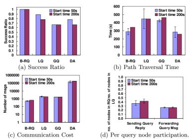
Fig. 6. Performance comparison in the absence of node failures.
